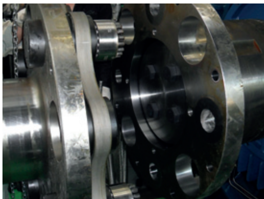
Lamidisc® SXJS-950 for marine test bench
