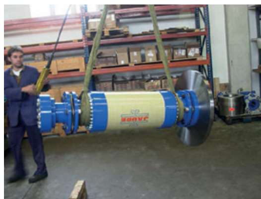
Lamidisc® with JGFS glass fiber shaft for wind industry
