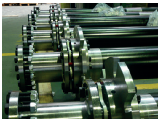
Lamidisc® 410-8 with locking device
