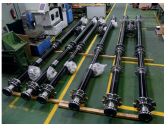
Lamidisc® 380-8 JHSS with hollow steel spacer and bearings
