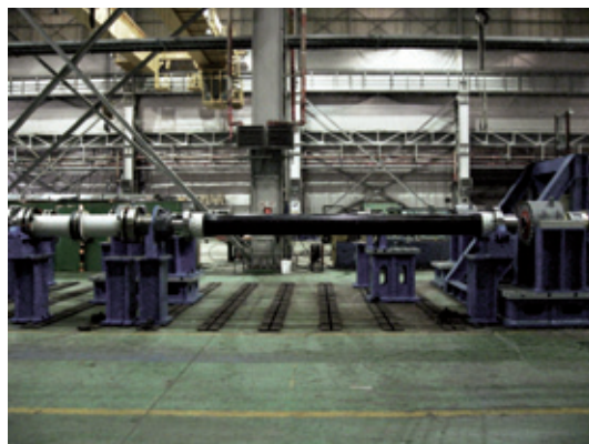
Lamidisc® 605-8 with JCFS composite shafts
