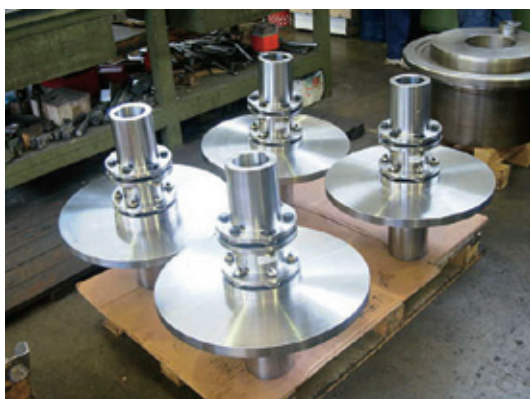
Lamidisc® SXRFD-202-6 with brake disc for cranes
