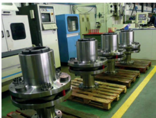
Lamidisc® SU-JS-730-6-JHC-230 with hydraulic coupling
