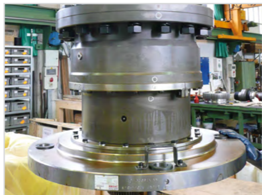
Shear pin type gear coupling
