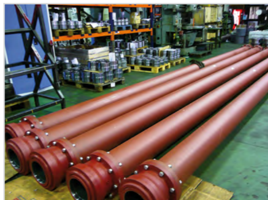
Jaure gear coupling for underwater operation
