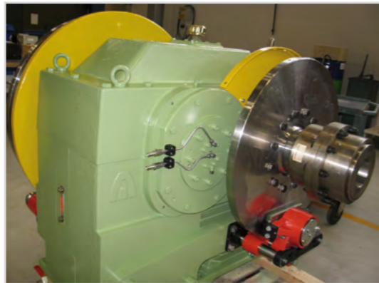
Jaure gear coupling with brake for hoisting
