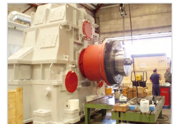
Jaure MTGX-HD-TI-1000 on wind test bench
