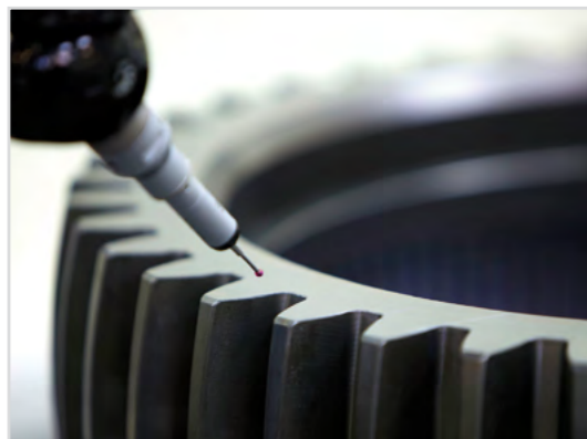
Gear inspection in CMM
