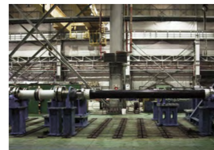
Carbon Fibre Shaft combined with LAMIDISC® coupling.
