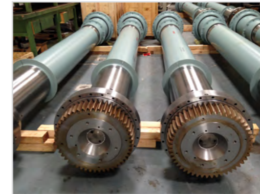
Case carburized gear spindles
