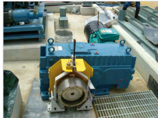
Disengaging gear with lever
